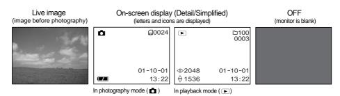
Each press of the DISP button switches the display in the following order (\* indicates default):
