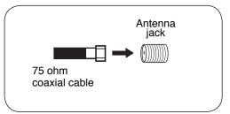
For basic cable service not requiring a converter/descrambler box, connect the Cable TV 75 ohm coaxial cable directly to the Antenna jack on the back of the TV/DVD.
