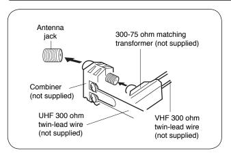
Connect the UHF 300 ohm twin-lead wire to the combiner (not supplied). Connect the VHF 300 ohm twin-lead wire to the 300-75 ohm matching transformer (not supplied). Attach the transformer to the combiner, then attach the combiner to the antenna jack on the back of the TV/DVD.
