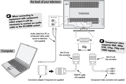
Connect the PC cable from the computer to the PC terminal on the back of the television.
