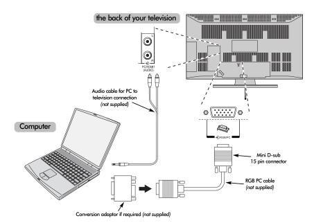
Connect the PC cable from the computer to the PC terminal on the back of the television.
