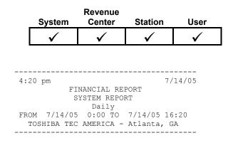
**Readings -** Non-resettable totals maintained by each POS station. This section prints if the USE NRGT option in System Setup/ System Config is set. These fields do not appear on the User Financial Report.
