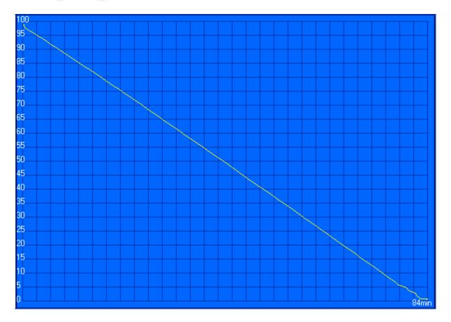
Well, the results speak for themselves. It took *84 minutes* for the battery to be fully depleted by Battery Eater 05. It also took *3 hours, 27 minutes and 51 seconds* for the battery to fully charge again.
