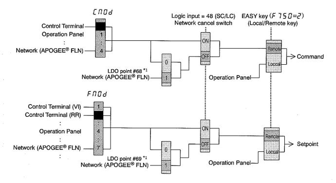
Be careful that  $[\Pi \square A]$  command and  $[\Pi \square A]$  setpoint are activated for a short time just after the inverter power turned on. Set  $[\Pi \square A]$  and  $[\Pi \square A]$  to "network" to prevent this problem.
