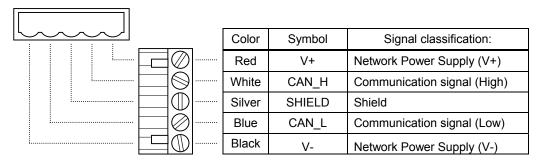
Size of connectable wire: 0.3 to 1.5mm<sup>2</sup> (AWG 22 to 16), Strip-off length: 7mm
