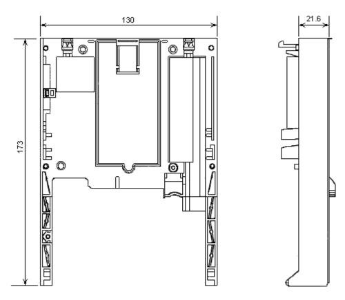
The control panel depth increases about 21.6mm when the option is installed. Secure the front space from the inverter control panel fully. The space which is necessary for the option installation varies in the inverter capacity rate. Please refer to the inverter instruction manual.
