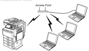
In the Infrastructure Mode, client computers can access to the equipment through a wireless network via an Access Point. The Infrastructure Mode is suitable for the wireless network that many client computers are connected at the same time. The Access Point will be required to establish the wireless network in the Infrastructure Mode.
