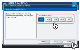
Select the low transmit power if you want to limit the area that the wireless communication is enabled. If you do not have to limit the area, select [100%].
