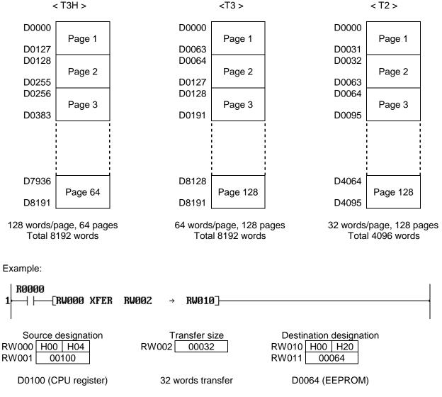
When R0000 is ON, 32 words data starting with D0100 is transferred to D0064 and after in the EEPROM. (Data write into EEPROM)
