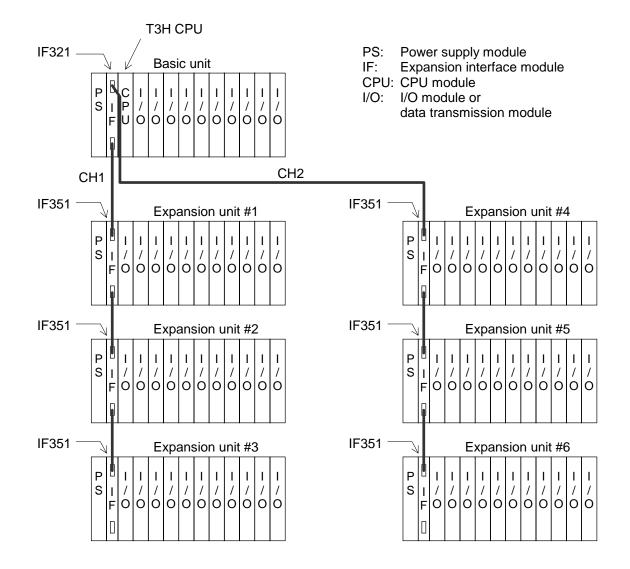
The figure below shows the T3H's maximum expansion configuration.
