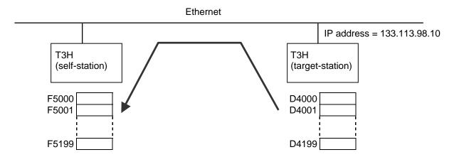
When R0030 is ON, 200 words data starting with D4000 of the T3H on which EN311 (IP address = 133.113.98.10) is installed, is read and stored in F5000 and after. When the operation is completed, the status is set in RW060 and instruction output comes ON.
