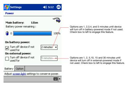
3 Select Option tab to adjust when battery alarm will come on, and to enable/disable Record and User programmable button wake up.
