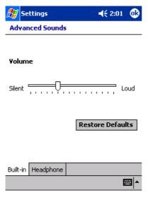
4 When using headphones, select the **Headphone** tab and make adjustments as shown in the figure below.
