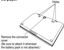
4 Turn the battery pack over and insert four catches into the player's corresponding holes ①. Then, slide the battery pack in the direction of the arrow ② until a "click" is heard.
