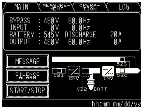
FIGURE 2.7.1 Main screen (Battery operation)
