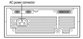
Rear view of the External Hard Drive Unit Z1
