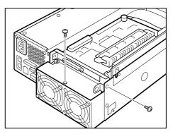
Fixing the PCI bracket
