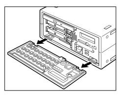
Removing the front panel
