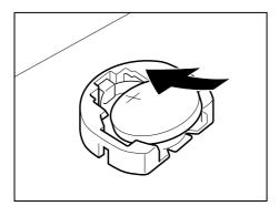
Installing the battery
