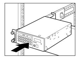
15 Insert the entire Base Assembly into the rack.
