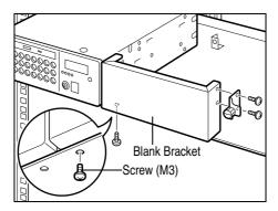
Fixing the Blank Bracket
