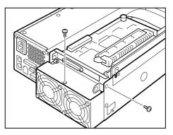
Fixing the PCI bracket
