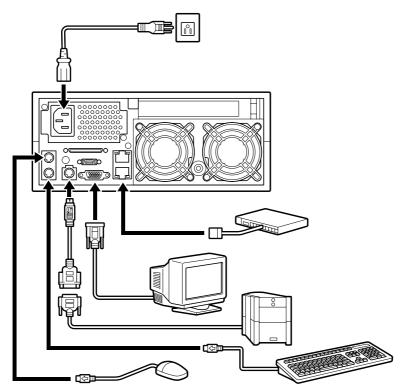
Connecting peripheral devices (Rear view)
