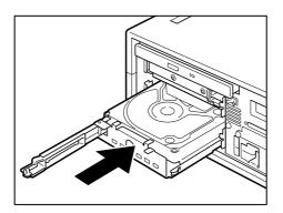
Installing the hard disk drive
