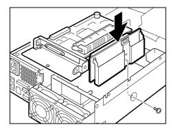
Installing the PCI riser card
