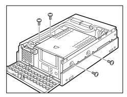
Installing the SCSI device
