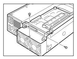
Fixing the PCI bracket
