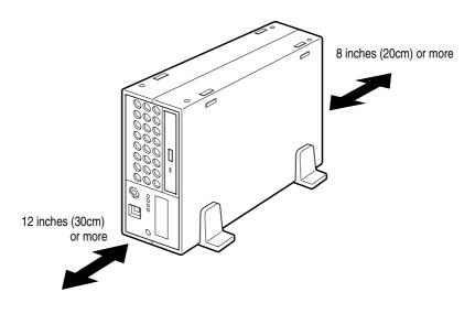
Minimum clearances required for vertical installation
