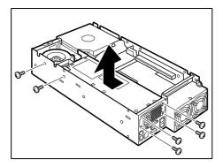
Lifting up the power supply unit.
