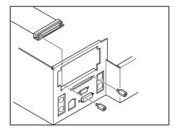
Installing the SCSI cable
