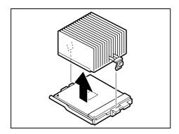
Removing the heat sink
