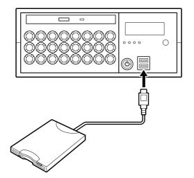
Connecting peripheral devices (Front view)
