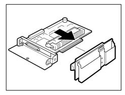
Inserting the expansion card
