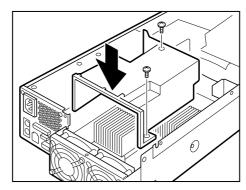
12 Attach the fan duct and fix it with two screws.
