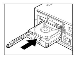
Installing the hard disk drive
