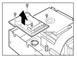
Removing the board for the wireless card
