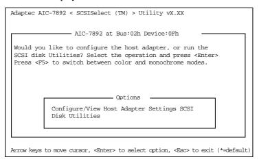
The internal SCSI drive are connected to the controllers. Only use the "Configure/View Host Adapter Setting" when the server is in the device setting screen mode. Do not modify the "SCSI Disk Utilities" setting.
