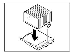
Attaching the heat sink
