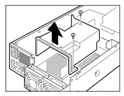
Removing the fan duct
