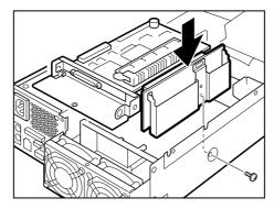
Installing the SCSI riser card
