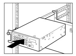
**12** Place the server bay on the Base Assembly and insert.
