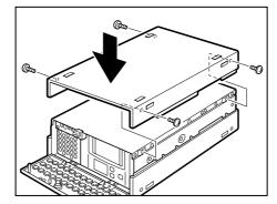
14 Attach the outer cover (upper) and fix it with four screws.
