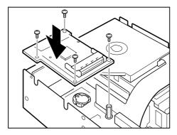
Installing the board for the wireless card
