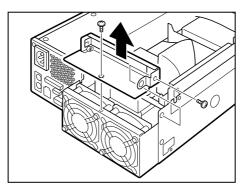
Removing the PCI bracket
