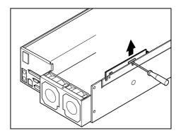
6 Remove two screws and the fan duct.
