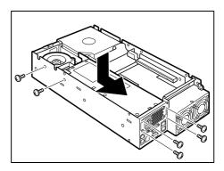
Installing the power supply unit
