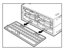
Removing the front panel
