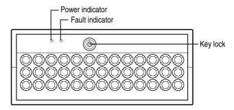
Front view with the front panel closed
