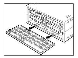
Removing the front panel
