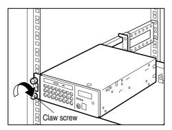
Fix the housing on the left and right
