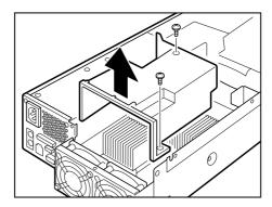
Removing the fan duct.
