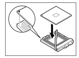
Inserting the CPU module
