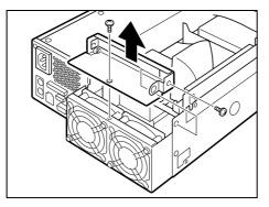
Removing the PCI bracket
