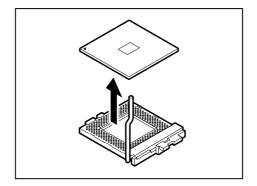
Removing the CPU module
