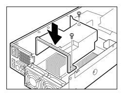
Installing the fan duct
