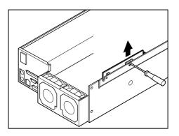
6 Remove two screws and the fan duct.
