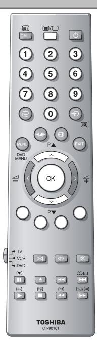
There are two *Modes*: **AUTO** will display **FASTEXT**, if available. **LIST** will display your four favourite pages. In either mode, as an alternative to the coloured buttons you can access a page by entering a 3-digit number, using the buttons on the remote control, or to advance to the next page, press the  $P \blacktriangle ( )$  button, to go back to the previous page press the  $P \blacktriangledown ( )$  button.
