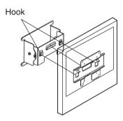
② By slightly lowering the LCD TV, you can hitch it on the hook
