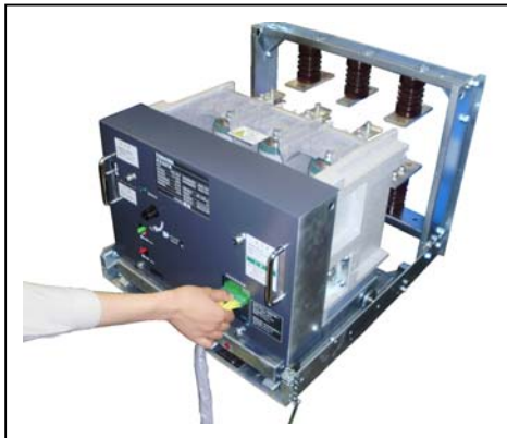
Figure 20 Insert the control circuit connector into the port on the VCB.
