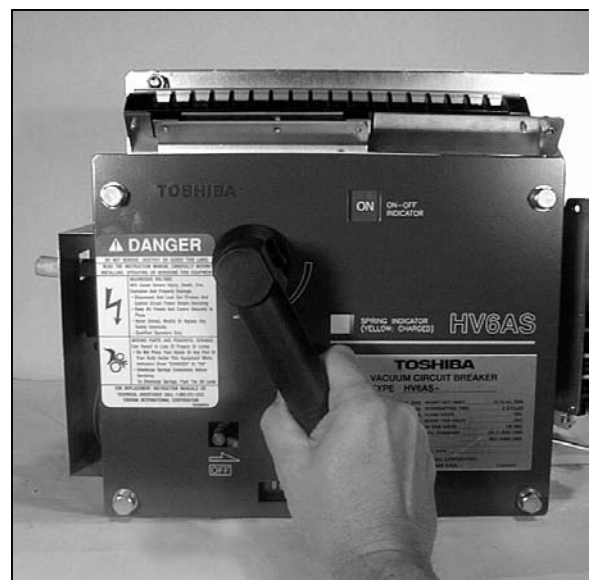
Fig. 24 Manually Closing Breaker
