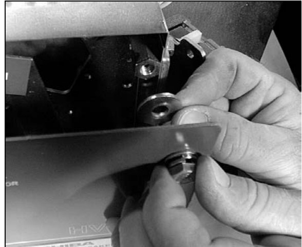
Fig. 10 Align Breaker With Panel Cutout
