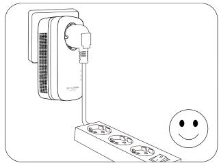
To take full advantage of the filter function of the Powerline Adapter and to improve data transmission in the network, always plug the multiple sockets into the integrated electrical socket of the Powerline Adapter.
