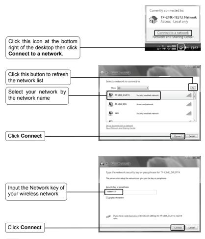
Note If you don't know the wireless network key, please consult the network administrator or log on to the setup page of your Wireless Router/Access Point with an Ethernet cable to check the wireless security settings. Please refer to the manual of your Wireless Router/Access Point or consult the manufactory's technical support for more details.
