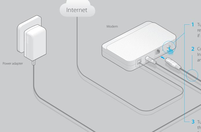
1 Turn off the modem and remove the backup battery if it has one.
