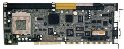
The HS-6038 is a 133MHz FSB Intel<sup>®</sup> 82815/82801BA chipset-based board designed for PICMG Bus Celeron<sup>™</sup>/Coppermine<sup>™</sup>/Tualatin<sup>™</sup> 800MHz~1.2GHz CPU compatibility. These features combine and make the HS-6038 an ideal all-in-one industrial single board computer. Additional features include an enhanced I/O with CompactFlash, VGA, dual LAN, audio, and two COM interfaces.
