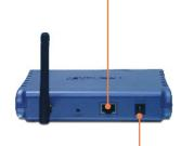
Connect the Power Adapter to the Access Point and then to a power outlet.
