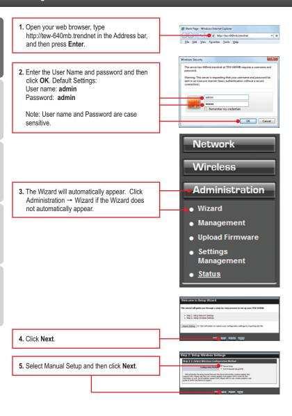
6. Select DHCP to have the TFW-640MB automatically obtain an IP address from your DHCP server (router). If Static IP address is selected you would need to configure the following:
