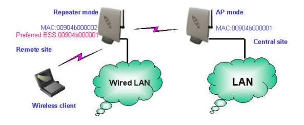
Wireless Bridge: This mode allows the connection of one or more remote LANs with a central LAN.
