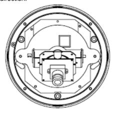
NOTE You can review the image quality from the Web browser when you complete the installation. If the image quality is poor, you have to disassemble the Dome cover to adjust the lens focus until the desired image appears clearly.
