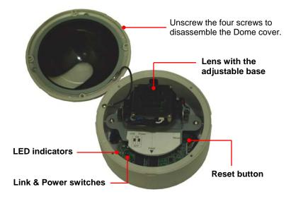
Reset button: Press the button to restart the camera.
