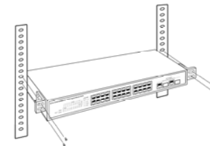
Figure 2. Mount the Switch in the rack
