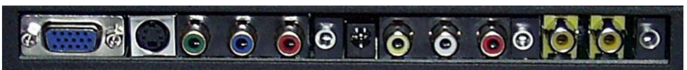
VGA S-Video Y Pb Pr PC 12V Video 1 L R Line Video Vdeo2 IR sound DC IN OUTPUT Ext.
