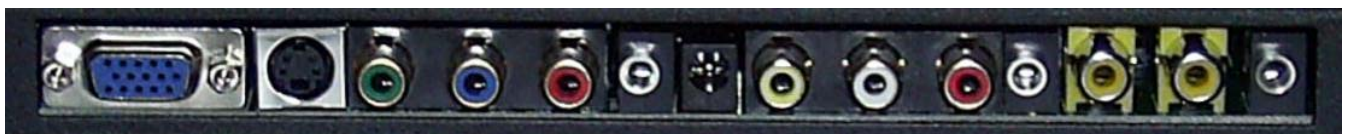
VGA S-Video Component Video 1 L R Line Video Vdeo2 IR OUTPUT Ext.
