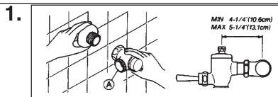
Install stop valve assembly (A) and wall flange. Refer to shown rough in dimension. Thread sealing compounds should be used on male NPT threads only.
