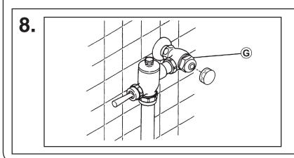
The stop cap screw cover should be replaced and tightly secured after final adjustments have been made.
