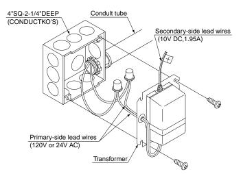
WARNING: Be sure to ground the 4"SQ box to eliminate the risk of electrical shock or fire hazard. Never kink or bend primary-side lead wires and/or secondary-side lead wires of the transformer when wiring them in the conduit tube or the junction box altogether.
