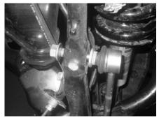
2. Using a 17mm ratchet, remove the nut from the bolt connecting the front sway bar link and the steering knuckle on both sides of the vehicle.
