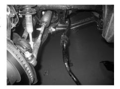
**6.** Using a 19 mm ratchet, remove the lower two ball joint bolts.
