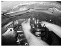
**7.** Remove the three upper strut mounting bolts with a 14 mm ratchet.
