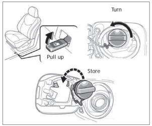
**NOTE:** If the cap is not tightened enough, the Check Engine "  $\bigcirc$  " indicator may illuminate.
