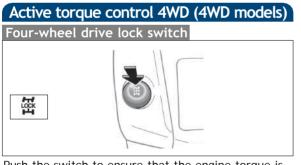
Push the switch to ensure that the engine torque is applied to the 4 wheels.
