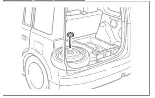
Loosen the bolt and remove it.
