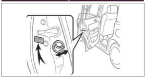
Move the lever to "LOCK," allowing the door to be opened only from the outside.
