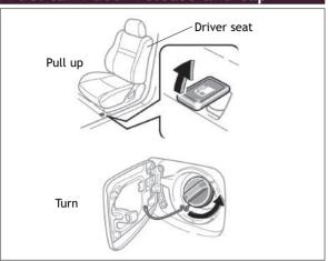
NOTE: If the cap is not tightened enough, Check Engine " indicator may illuminate.
