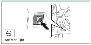
Designed to provide warning when tire pressure of any one of the tires is critically reduced while the vehicle is moving. It must be re-initialized by pushing and holding the " SET" button if indicator light blinks twice every second, and/or after replacing or rotating tires or wheels.
