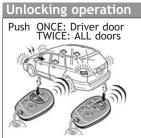
NOTE: After unlocking, if a door is not opened within thirty (30) seconds, all doors will relock for safety.
