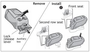
The console box can be removed and installed between the front or second row seats.
