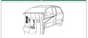
Move the lever to "LOCK," allowing the sliding door to be opened only from the outside.
