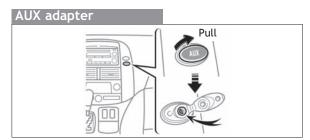
By inserting a mini plug of a commercially available component into the AUX adapter, you can listen to music from a portable audio device through the vehicle's speaker system.
