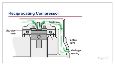
When the pressure within the cylinder exceeds the discharge (or head) pressure, the discharge valve is forced open, allowing the compressed refrigerant vapor to leave the cylinder. The compressed refrigerant travels through the headspace and leaves the compressor through the discharge opening.
