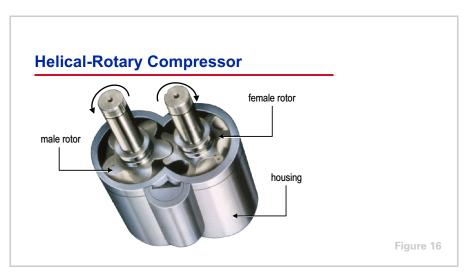
The rotors are meshed and fit, with very close tolerances, within the compressor housing. The gap between the two rotors is sealed with oil, preventing the compressed refrigerant vapor from escaping through the mating surfaces.
