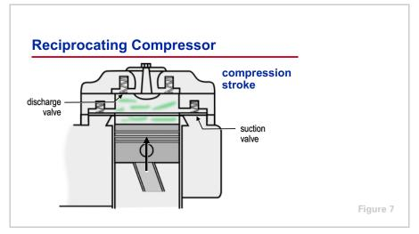
During the **compression stroke**, the piston reverses its direction and travels toward the discharge valve, compressing the refrigerant vapor and increasing the pressure within the cylinder. When the pressure inside the cylinder exceeds the suction pressure, the suction valve is forced closed, trapping the refrigerant vapor inside the cylinder.
