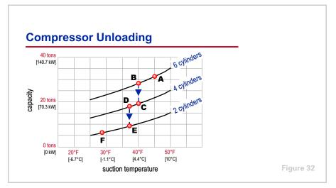
At design conditions, the capacities of the evaporator coil and compressor balance (**A**) at a suction temperature of  $45 \,^{\circ}$ F [7.2 $\,^{\circ}$ C] and a capacity of 31 tons [109 kW]. As the cooling load decreases below this balance point, assuming a constant condensing pressure, the compressor pumping capacity decreases with the falling suction temperature along the six-cylinder curve until it reaches **B**. Here, the compressor unloads the first set of two cylinders.
