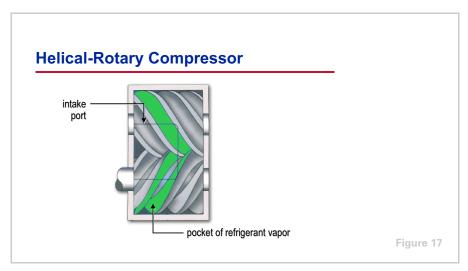
Refrigerant vapor enters the compressor housing through the **intake port** and fills the pockets formed by the lobes of the rotors. As the rotors turn, they push these pockets of refrigerant toward the discharge end of the compressor.
