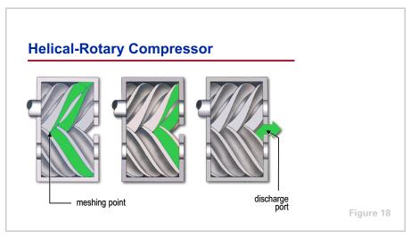
Viewing the compressor from the opposite side shows that continued rotation of the meshed rotor lobes drives the trapped refrigerant vapor (to the right), toward the discharge end of the compressor, ahead of the meshing point. This action progressively reduces the volume of the pockets, compressing the refrigerant.
