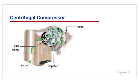
In this example centrifugal compressor, refrigerant vapor is drawn into the compressor and enters the center of impeller. This particular centrifugal compressor uses multiple impellers to perform the compression process in stages. The impellers rotate on a common shaft that is connected to the motor.
