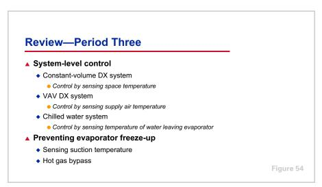
Period Three considered the entire system and discussed how the capacity of the compressor is controlled to maintain desired space conditions.
