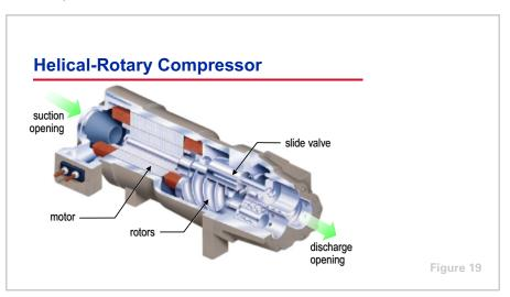
In this example helical-rotary compressor, refrigerant vapor is drawn into the compressor through the suction opening and passes through the motor, cooling it. The refrigerant vapor is drawn into the compressor rotors where it is compressed and discharged out of the compressor.
