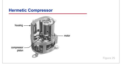
A **hermetic compressor**, on the other hand, seals the motor within the compressor housing. This motor is cooled by the refrigerant, either by refrigerant vapor that is being drawn into the compressor from the suction line or by liquid refrigerant that is being drawn from the liquid line. The heat from the motor is then rejected by the condenser.
