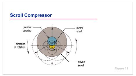
The center of the scroll journal bearing and the center of the motor shaft are offset. This offset imparts an orbiting motion to the driven scroll. Rotation of the motor shaft causes the scroll to orbit—not rotate—about the shaft center.
