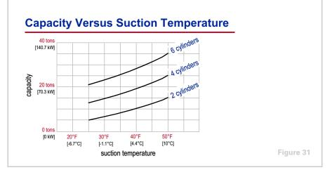
A plot of compressor capacity versus suction temperature (assuming a constant condensing temperature) reveals that the capacity of the compressor increases as the suction temperature increases. As the suction temperature, and, therefore, the suction pressure, increases, the refrigerant vapor becomes denser. A greater quantity of refrigerant can be compressed in a given compression cycle and the capacity of the compressor is higher.
