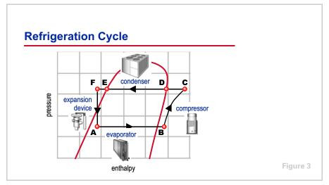
The **pressure-enthalpy** (**P**-*h*) **chart** plots the properties of a refrigerant: refrigerant pressure (vertical axis) versus enthalpy, or heat content (horizontal axis). A diagram of the basic vapor-compression refrigeration cycle can be superimposed on a pressure-enthalpy chart to demonstrate the function of each component in the system.
