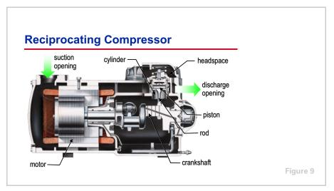
In the reciprocating compressor shown, the refrigerant vapor from the suction line enters the compressor through the suction opening. It then passes around and through the motor, cooling the motor, before it enters the cylinder to be compressed. The compressed refrigerant leaves the cylinder, travels through the headspace, and leaves the compressor through the discharge opening.
