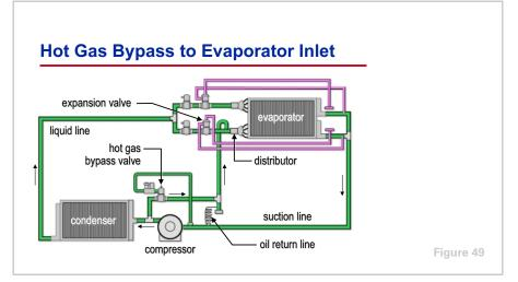
Hot gas bypass may be another solution for preventing evaporator frosting in DX applications. Hot gas bypass diverts hot, high-pressure refrigerant vapor from the discharge line to the low-pressure side of the refrigeration system. This added "false load" helps to maintain an acceptable suction pressure and temperature. Hot gas bypass, however, fails to reduce energy consumption because it does not allow the compressor to shut off at these low load conditions.
