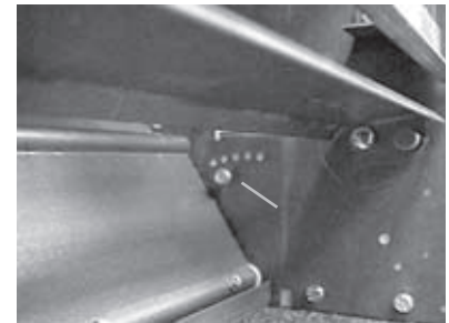
Figure 30. Re-locate the damper stop screw to adjust the damper position. The factory positions the stop screw in the 25% open position.
