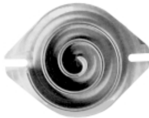
One of two matched scroll plates — the distinguishing feature of the scroll compressor.
