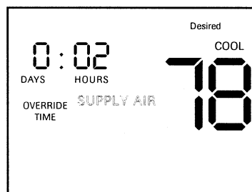
Figure I-P-6. Temporary manual override menu screen
