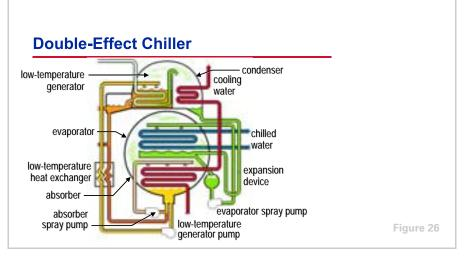
Next, the refrigerant travels through the condenser, expansion device, evaporator and absorber in a manner similar to refrigerant travel in the singleeffect absorption chiller.
