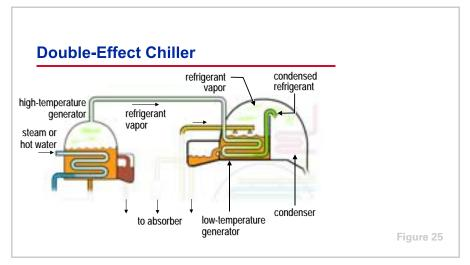
In the **high-temperature generator**, very high temperature steam or hot water flows through tubes that are immersed in an absorbent solution that is at an intermediate concentration. The solution absorbs heat from the warmer steam or water, causing the refrigerant to boil and separate from the absorbent solution. As the refrigerant boils away, the absorbent solution becomes concentrated and returns to the absorber.
