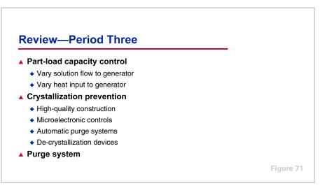
Period Three explained the part-load operation of the absorption chiller. It described the use of energy valves, burner controls, throttling and bypass valves, and adjustable-frequency drives as methods for controlling the capacity on the chiller. Valves and AFDs are used to vary the flow rate of solution to the generator. Modulating energy valves and burner controls are used to vary the heat input to the generator.
