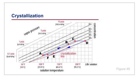
By plotting the single-effect absorption refrigeration cycle on the equilibrium chart, it is apparent that crystallization is most likely to occur in the heat exchanger. At this particular condition, the 65% concentrated solution (**D**) is cooled to 135°F [57.2°C] (**E**) as it passes through the heat exchanger. As noted previously, the saturation temperature of 65% solution is 123°F [50.6°C] so there is no danger of crystallization.
