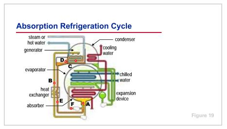
A diagram of a typical absorption refrigeration cycle can be superimposed on this equilibrium chart to demonstrate the function of each component in the system.
