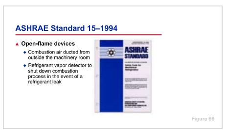
In general, ASHRAE Standard 15-1994, "Safety Code for Mechanical Refrigeration," does not apply to absorption water chillers due to Section 2.3, which states:
