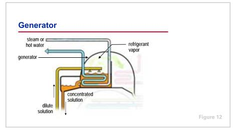
Starting on the high-pressure side of the cycle, the purpose of the **generator** is to deliver the refrigerant vapor to the rest of the system. It accomplishes this by separating the water (refrigerant) from the lithium bromide-and-water solution.
