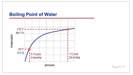
At a given pressure, the temperature at which a liquid will boil into a vapor is the same temperature at which the vapor will condense back into a liquid. This curve illustrates the pressures and corresponding temperatures at which water (the refrigerant) boils and condenses.
