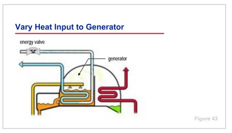
In order to vary the solution concentration, absorption chillers vary the heat input to the generator. This figure shows a modulating energy valve on a single-effect, steam absorption chiller. At part load, in response to a changing leaving-chilled-water temperature, the energy valve begins to close, reducing the amount of heat input to the generator. Similarly, on a direct-fired absorption chiller, the amount of heat input to the generator is varied by modulating the capacity of the burner.
