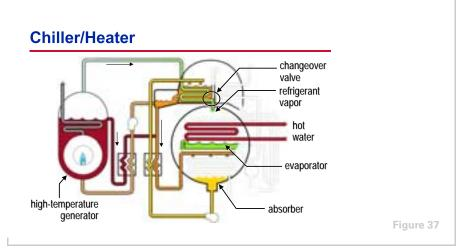
An alternate method is to use the evaporator as a condenser in the heating mode. In this example chiller, by switching the cooling/heating changeover valve the chiller switches to heating mode, and hot water can be delivered using the same piping system that was used to supply chilled water in the cooling mode. The cooling tower and refrigerant pumps can typically be shut off.
