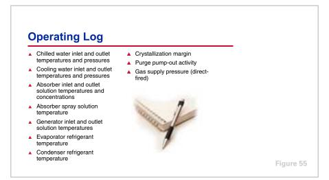
Chiller operation should be checked daily and recorded in an operating log. Standard operating logs include: solution data; evaporator, absorber, and
