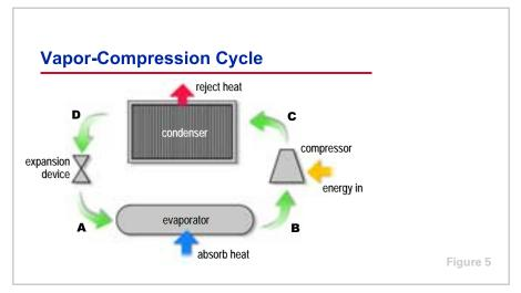
In the vapor-compression refrigeration cycle, refrigerant enters the evaporator in the form of a cool, low-pressure mixture of liquid and vapor ( $\mathbf{A}$ ). Heat is transferred from the relatively warm air or water to the refrigerant, causing the liquid refrigerant to boil. The resulting vapor ( $\mathbf{B}$ ) is then pumped from the evaporator by the compressor, which increases the pressure and temperature of the refrigerant vapor.
