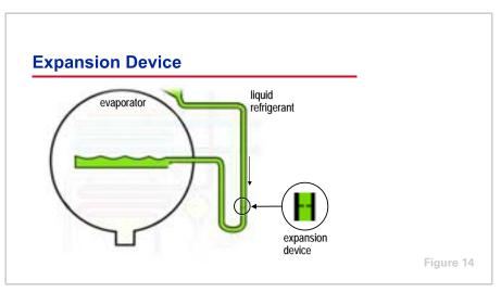
From the condenser, the liquid refrigerant flows through an **expansion device** into the evaporator. The expansion device is used to maintain the pressure difference between the high-pressure (condenser) and low-pressure (evaporator) sides of the refrigeration system. In this example, the expansion device is a throttling pipe, which is a long section of pipe with an orifice restriction in it. It creates a liquid seal that separates the high-pressure and lowpressure sides of the cycle.
