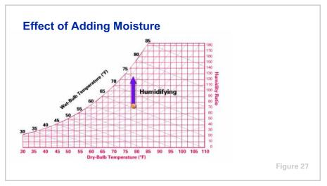
On the other hand, if moisture is added to air without changing the dry-bulb temperature, the air condition moves upward along a dry-bulb temperature line.
