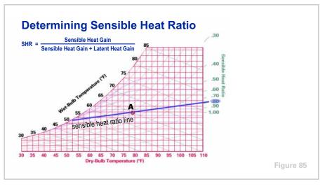
In Period Three, the **ratio of sensible heat gain to total heat gain** was discussed. With the aid of the sensible heat ratio scale on the chart, an SHR line was drawn. It was also shown that any combination of air conditions that fall on this line will maintain the desired room conditions **A**. Each set of conditions requires a different supply airflow.
