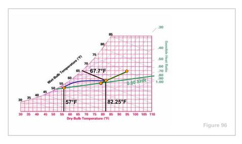
**e** Airflow (cfm) =  $\frac{156,000 \text{ Btu/hr}}{1.085 \times (78^{\circ}\text{F} - 57^{\circ}\text{F})} = 6,847 \text{ cfm}$
