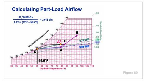
At part load, when the SHR of the room is reduced from 0.80 to 0.70, the VAV system responds by reducing the quantity of 56.5°F air supplied to the room to match the reduced sensible heat gain. The part-load sensible heat gain of 47,000 Btu/hr and the constant supply air temperature, 56.5°F DB, are used to determine the required part-load air quantity.
