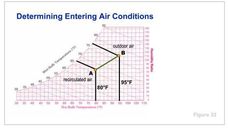
If outdoor air **B** is mixed with recirculated air **A**, the conditions of the resulting mixture are found somewhere on a straight line connecting the two points.
