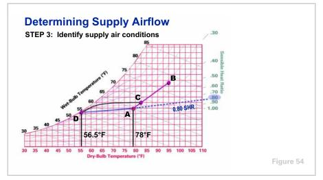
The third step is to determine the required supply air conditions. This is where the coil curves are used. Using the curvature of the nearest coil line as a guide, draw a curve from the mixed-air condition  $\mathbf{C}$  until it intersects the SHR line.
