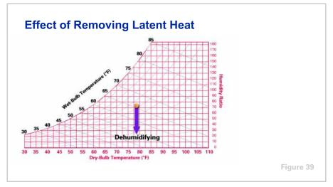
Conversely, if only latent heat is removed, the line moves vertically downward along a constant dry-bulb temperature line. This results in a lower moisture content or humidity ratio.
