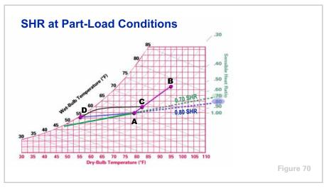
To maintain the design room conditions **A** for this part-load sensible heat ratio, a different supply air condition—one that falls on the 0.70 SHR line—and a different airflow are required. But suppose the system in this example was designed to deliver a constant quantity of air and vary its supply temperature to meet the changing loads.
