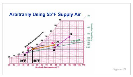
Plotting this new SHR line on the psychrometric chart, we find that the SHR line crosses the coil curve at approximately  $49^{\circ}$ F DB (**D**).
