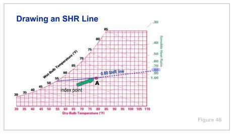
Assume that room design conditions (**A**) are  $78\,^{\circ}$ F DB and  $65\,^{\circ}$ F WB, and that the sensible heat ratio is calculated as 0.80. That is, sensible heat gain represents 80% of the total (sensible plus latent) heat gain.
