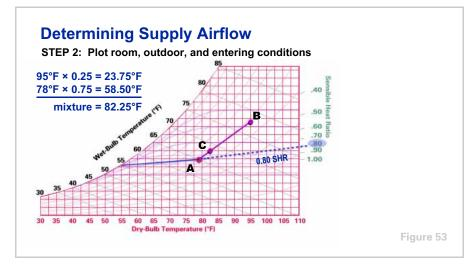
Plot the outdoor air **B** (95°F DB, 78°F WB) and indoor air **A** (78°F DB, 65°F WB) conditions on the psychrometric chart. Then calculate the mixed-air conditions using the method learned in Period 2.
