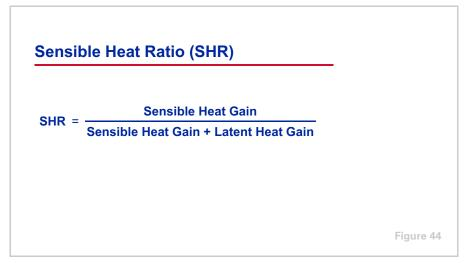
The sensible heat ratio, abbreviated as SHR, refers to the comparison of sensible heat gain to total heat gain (sensible heat plus latent heat). Once this ratio is known, an SHR line can be drawn on the psychrometric chart.
