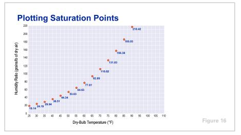
These saturation points can be plotted on a chart with dry-bulb temperature along the horizontal axis and humidity ratio along the vertical axis.
