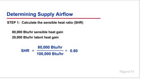
To demonstrate how the required supply airflow is determined, assume that a room's sensible heat gain is 80,000 Btu/hr and its latent heat gain is 20,000 Btu/hr. First, divide the sensible heat gain by the total heat gain. The resulting sensible heat ratio (SHR) is 0.80.
