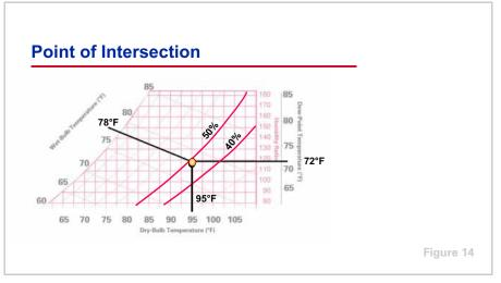
Only one point on the psychrometric chart represents air with both of these conditions. This point is located where the vertical 95°F dry-bulb (DB) and diagonal 78°F wet-bulb (WB) temperature lines intersect.
