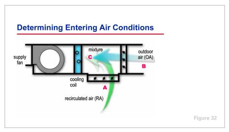
The air entering the cooling coil may be 100% recirculated (**A**), 100% outdoor (**B**), or a mixture of the two (**C**).
