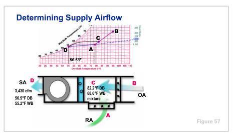
The cooling coil must cool and dehumidify 3,430 cfm of air from the entering condition **C** to the supply air condition **D** to maintain the desired room conditions.
