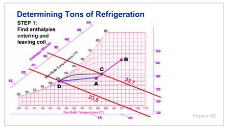
Using the previous example for calculating supply airflow, the first step is to determine the enthalpies of the air entering and leaving the cooling coil. This is accomplished by lining up three points on the chart, including the entering-air condition and identical points on the two enthalpy scales—one each on the left and right edges of the psychrometric chart.
