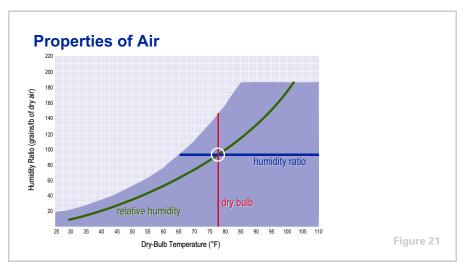
This basic chart now shows three air conditions: dry-bulb temperature (vertical lines), humidity ratio (horizontal lines) and relative humidity (diagonally curved lines).
