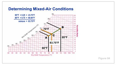
In Period Two, a method was discussed to determine the resulting properties of an air mixture. By plotting the conditions of the **outdoor air** and **recirculated air**, and using the percentage of outdoor air, the resulting condition of the air mixture was calculated and plotted on a straight line from **A** to **B** connecting the two air conditions.
