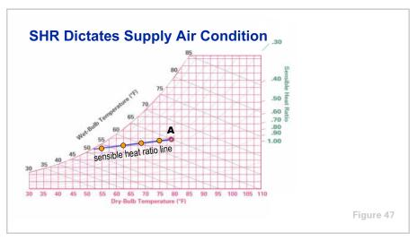
Supply air with any combination of dry-bulb and wet-bulb temperatures that falls on this line will be able to absorb the room's sensible and latent heat in the correct proportions needed to maintain the desired room conditions ( $\mathbf{A} = 78^{\circ}$ F DB, 65°F WB).
