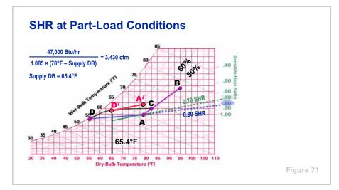
In response to the reduction in room sensible heat gain, the coil capacity is throttled, raising the supply air temperature from D to D' to balance the new room sensible heat gain. This new supply air temperature is dictated by the equation:
