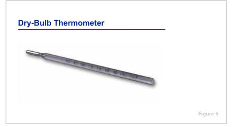
**Dry-bulb temperatures** are read from an ordinary thermometer that has a dry bulb.
