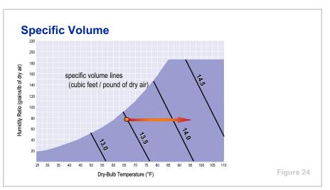
There is one more property of air that is displayed on the psychrometric chart specific volume. **Specific volume** is defined as the volume of one pound of dry air at a specific temperature and pressure. As one pound of air is heated it occupies more space—the specific volume increases.
