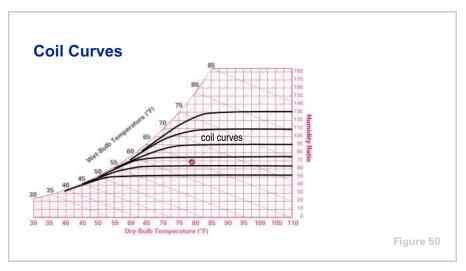
Before proceeding, one more set of curves on the psychrometric chart must be identified. These curved lines represent the changes in dry-bulb and wet-bulb temperatures as air passes through a "typical" cooling coil. These are commonly referred to as **coil curves**; they depict approximate coil performance. Exact coil performance depends on the actual coil geometry and can be precisely determined by coil selection software.
