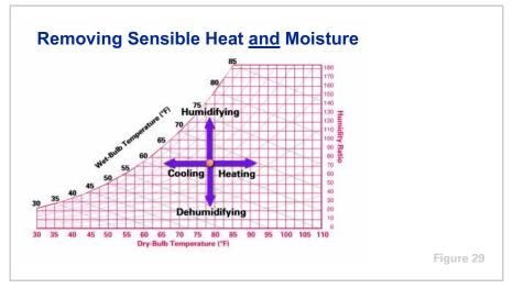
Put all of these changes together on one chart and they show the direction the air condition will move when the dry-bulb temperature or moisture content is altered.
