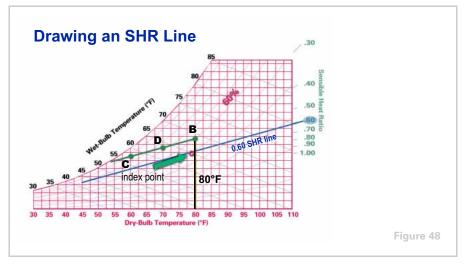
Sensible-heat-ratio lines for other conditions are drawn in the following manner. Assume that room design conditions are 80°F DB and 60% RH, and that the SHR is calculated as 0.60.
