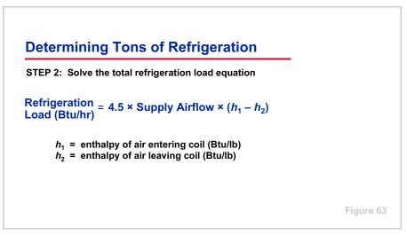
The total refrigeration load, in terms of Btu per hour, is then calculated using the following formula, where the supply airflow is expressed in cfm,  $h_1$  is the entering-air enthalpy in Btu/lb, and  $h_2$  is the leaving-air enthalpy in Btu/lb.
