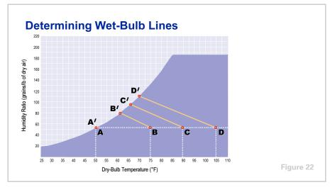
To complete this basic chart, the wet-bulb temperature lines must be added.
