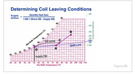
After determining the entering air conditions for the coil and the slope of the SHR line, the **coil curves** were used to find the required supply air conditions. This point (**D**) was established by the intersection of the coil curve and the SHR line.
