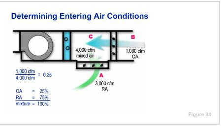
In this example, 1,000 cfm of outdoor air (OA) is mixed with 3,000 cfm of recirculated air (RA) for a total supply airflow of 4,000 cfm.
