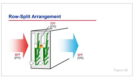
Row-split coils are very difficult to split into equal-capacity sections. Since the air entering the downstream section of coil has already been cooled somewhat by the upstream section of coil, the air-to-refrigerant temperature difference is much smaller. Therefore, the downstream section of coil requires more rows of tubes to deliver about the same capacity as the upstream section of coil. A common row-split arrangement uses two rows for the upstream section and
