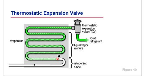
In addition to maintaining a pressure difference, the **thermostatic expansion valve** controls the quantity of liquid refrigerant entering the evaporator. It ensures that the refrigerant will be completely vaporized within the evaporator (**A**) and maintains the proper amount of superheat in the system.
