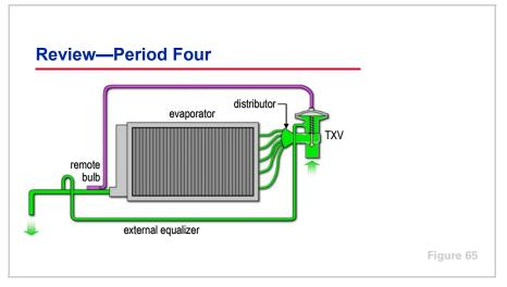
Period Four reviewed the operation of the expansion device, specifically the thermostatic expansion valve. The expansion device is used to maintain the pressure difference between the high-pressure (condenser) and low-pressure (evaporator) sides of the system established by the compressor.
