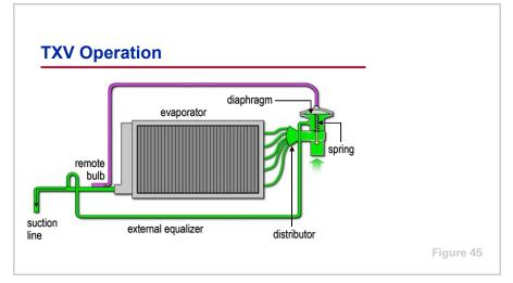
In a typical TXV application, the outlet of the valve is connected to the distributor. A remote bulb is attached to the suction line, where it senses the refrigerant vapor temperature leaving the evaporator. This bulb is charged with refrigerant and as heat is transferred from the suction line to the bulb, the refrigerant inside the bulb vaporizes. The resulting refrigerant vapor pressure is transmitted through a tube to the space above a diaphragm in the TXV.
