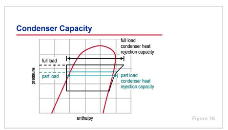
As the system load decreases, the heat rejection capacity of the condenser is greater than the load. Because of this excess capacity, the condenser matches the decreasing load by operating at progressively lower pressures. Additionally, a reduction in outdoor air temperature allows the temperature of the air or water flowing through the condenser to drop. This also has the effect of lowering the condensing pressure.
