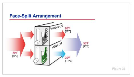
At lower loads, only one section of the face-split coil is active. A portion of the air passes through the active lower section and is cooled, while the rest of the air passes through the inactive top section and remains unconditioned. The two airstreams mix downstream of the coil, producing average temperature and humidity conditions. At higher loads, both sections of the coil are activated, providing a more uniform leaving-air temperature.
