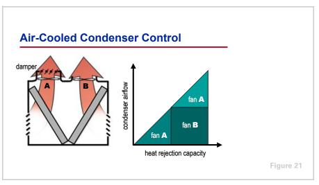
A common method of controlling the capacity of an air-cooled condenser is to vary the airflow across the condenser coil. The heat-rejection rate of a multiplefan condenser is often controlled by cycling fans on and off to maintain acceptable condensing pressures. Alternatively, the airflow across the coil can be varied by using a damper or a variable-speed drive on one or more of the fans.
