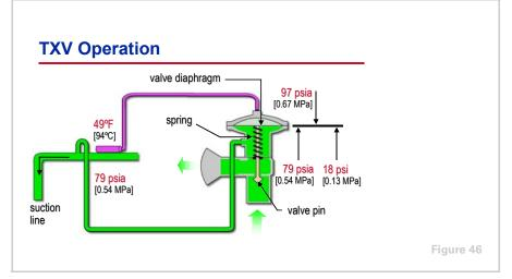
Using the conditions from the previous example, the 49°F [9.4°C] refrigerant vapor leaving the evaporator boils the refrigerant in the bulb, generating 97 psia [0.67 MPa] of pressure within the remote bulb. This pressure is transmitted to the top side of the valve diaphragm, creating a force that pushes down on the diaphragm.
