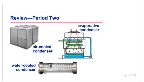
Period Two discussed the different types of condensers and methods of condenser control. The condenser rejects heat from the refrigerant to air, water, or some other fluid. The three common types of condensers are air-cooled, water-cooled, and evaporative.
