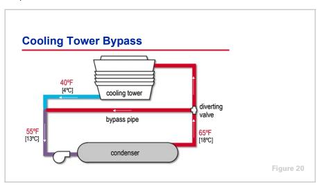
Another example is a system that must start and operate during cooler weather. The cold tower water would force the condensing pressure down to the point where the system could not operate. In this example, the temperature of the water entering the condenser is controlled by a diverting valve and a coolingtower bypass pipe.
