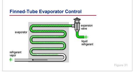
Typically, an expansion valve is used to control the flow rate of refrigerant through the evaporator to maintain the proper amount of superheat, ensuring that the liquid refrigerant will be completely vaporized. Working in conjunction with the unloading or cycling compressors, the expansion valve allows the evaporator capacity to match the system load. The operation of the expansion valve will be discussed further in Period Four.
