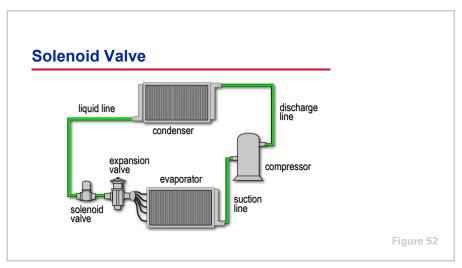
Another common use of a solenoid valve is to enable system pump-down and prevent the refrigerant from migrating through the system when the compressor is shut off. In this application, a single solenoid valve is installed in the liquid line, upstream of all expansion valves.
