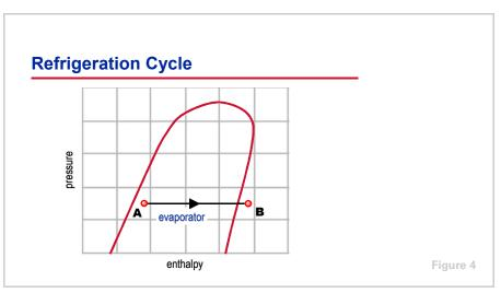
A diagram of a typical vapor-compression refrigeration cycle can be superimposed on a pressure-enthalpy (P-*h*) chart to demonstrate the function of each component in the system. The **pressure-enthalpy chart** plots the properties of a refrigerant – refrigerant pressure (vertical axis) versus enthalpy (horizontal axis). **Enthalpy** is a measure of the heat content, both sensible and latent, per pound [kg] of refrigerant.
