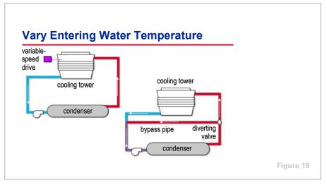
Another method of controlling the capacity of a water-cooled condenser is to vary the temperature of the water entering the condenser.
