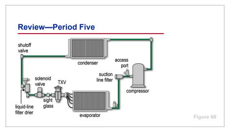
Period Five discussed several accessories commonly used in comfort-cooling applications, including: solenoid valve, liquid-line filter drier, moisture-indicating sight glass, suction line filter, hot gas muffler, shutoff valve, and access port.
