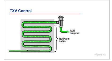
On the other hand, if too much liquid refrigerant enters the evaporator, not all of it will be vaporized. As a result, some liquid refrigerant gets into the compressor suction line. Since the compressor is designed to compress vapor and not liquid, liquid refrigerant can cause excess wear and damage to the compressor.
