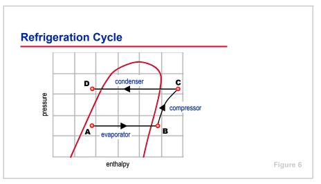
Within the condenser, heat is transferred from the hot refrigerant vapor to relatively cool ambient air or cooling water. This reduction in the heat content of the refrigerant vapor causes it to desuperheat, condense into liquid, and further subcool before leaving the condenser ( $\mathbf{D}$ ) for the expansion device.
