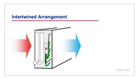
The **intertwined** coil configuration splits the coil sections by alternating the tubes fed in each row between two distributors.
