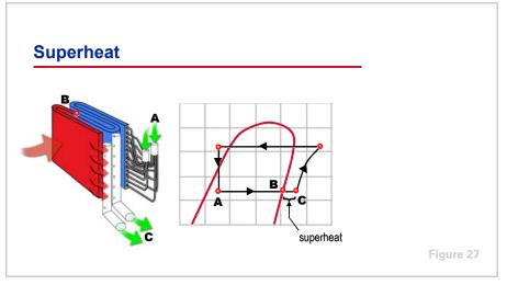
Inside the final length of tubes the location where the temperature difference between the refrigerant and the air is highest this larger temperature difference accelerates the rate of heat transfer and the refrigerant vapor absorbs even more heat. When the liquid refrigerant has completely evaporated, this additional heat gain to the vapor is called **superheating**.
