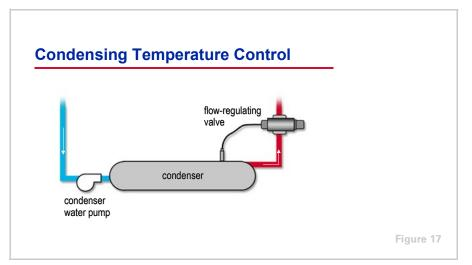
One common method of controlling the capacity of a water-cooled condenser is to vary the rate at which water flows through the condenser.
