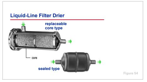
A typical liquid-line filter drier includes a molded, porous core. The core has a high affinity for moisture and removes foreign matter from the refrigerant.
