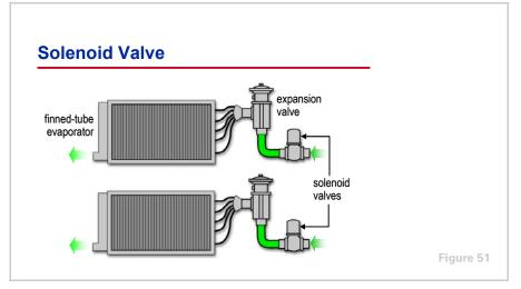
One common use of a solenoid valve is to control the flow of liquid refrigerant to multiple sections of the evaporator. In this application, a valve is installed in the liquid line, upstream of the expansion valve for each individually controlled section of the evaporator coil.
