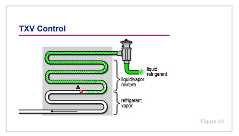
If not enough liquid refrigerant enters the evaporator, it vaporizes too quickly (**A**). As a result, the remaining coil tubes fill with vapor, producing very little refrigeration effect.
