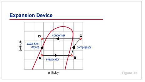
An **expansion device** is used to maintain a pressure difference between the high-pressure (condenser) and low-pressure (evaporator) sides of the system established by the compressor. This pressure difference allows the evaporator temperature to be low enough to absorb heat from the air or water to be cooled, while also allowing the refrigerant to be at a high enough temperature in the condenser to reject heat to air or water at normally available temperatures.
