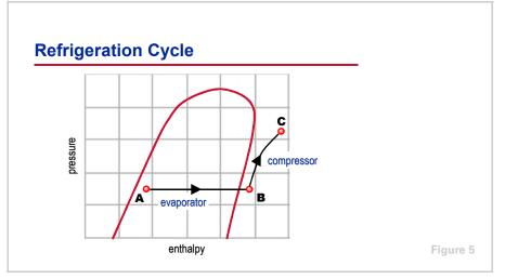
The compressor draws in the superheated refrigerant vapor (**B**) and compresses it to a pressure and temperature (**C**) high enough that it can reject heat to another fluid. This hot, high-pressure refrigerant vapor then travels to the condenser.
