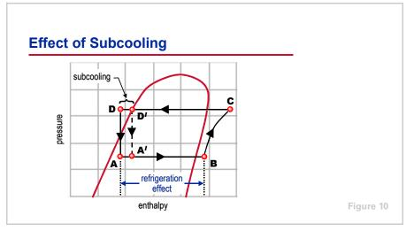
The benefit of subcooling on system performance can be demonstrated by comparing the performance of a system with and without subcooling.
