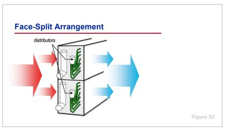
When an evaporator contains more than one liquid-refrigerant distributor, it is split into independently-controlled sections, each being served by its own expansion valve. By turning on and shutting off these coil sections, the evaporator can further control its capacity to better match the system load.
