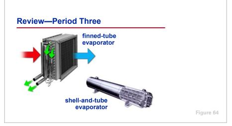
Period Three presented the different types of evaporators and methods of evaporator control. The evaporator transfers heat from air, water, or some other fluid to the cool liquid refrigerant. The two common types of evaporators are finned-tube and shell-and-tube.
