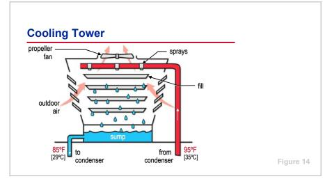
A **cooling tower** is a device commonly used to cool condensing water. In this design, warm water is sprayed over the fill inside the cooling tower while a propeller fan draws outdoor air upward through the fill. The movement of air through the spray causes some of the water to evaporate, a process that cools the remaining water. This cooled water then falls to the tower sump to be returned to the condenser.
