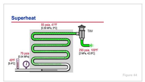
Continuing with this example, the refrigerant enters the evaporator coil at 85 psia [0.59 MPa] and 41°F [5°C]. Assuming that the pressure drop through the coil tubes is 6 psi [0.04 MPa], the refrigerant vapor leaves the coil at 79 psia [0.54 MPa]. The temperature gauge at the outlet of the evaporator coil indicates that the superheated refrigerant vapor leaves at 49°F [9.4°C].
