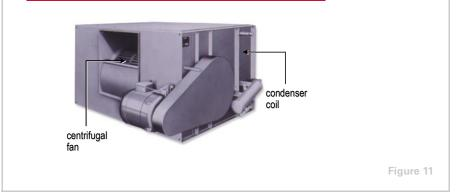
An alternative air-cooled condenser uses a centrifugal fan to draw or blow air over the condensing coil. The principal advantage of this design is that the centrifugal fan is capable of overcoming the higher static-pressure losses associated with ductwork. Therefore, if the condenser is to be located indoors and uses a duct system to deliver air to and from the condenser coil, the **centrifugal fan air-cooled condenser** is probably best suited for this application.
