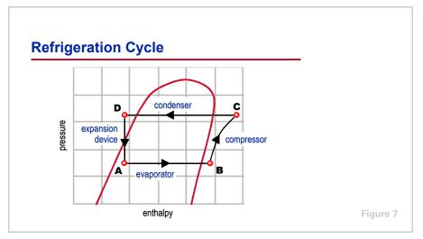
Finally, the high-pressure liquid refrigerant (**D**) flows through the expansion device, causing a large pressure drop that reduces the pressure of the refrigerant to that of the evaporator. This pressure reduction causes a small portion of the liquid to boil off, or flash, cooling the remaining refrigerant to the desired evaporator temperature.
