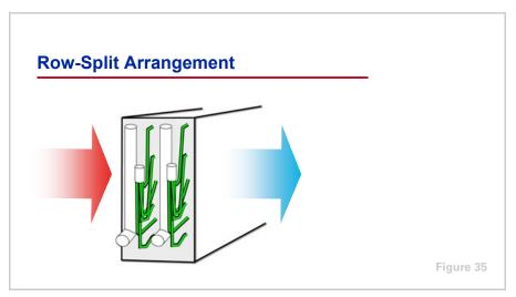
Finally, the **row-split** coil configuration, also called vertical-split or series-flow, places the independently-controlled coil sections in series in the airstream. All of the air passes through both coil sections, one before the other.
