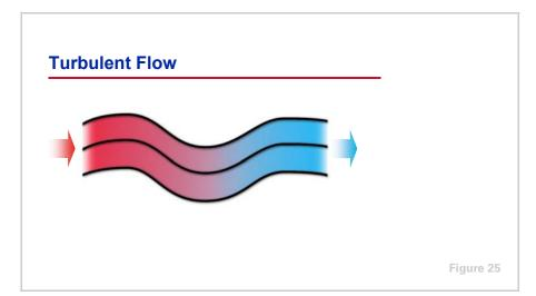
The fins of the coil are formed to produce turbulence as the air passes through them. This turbulence enhances heat transfer, preventing stratification within the coil-leaving airstream.
