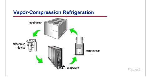
The major components of a vapor-compression refrigeration system include the compressor, condenser, expansion device, and evaporator. The latter three will be discussed in this clinic – the compressor is discussed in a separate clinic.
