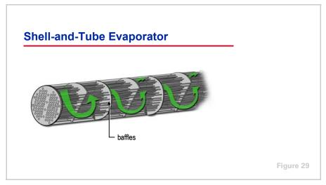
Baffles within the shell direct the water in a rising and falling flow path over the tubes that carry the refrigerant. This results in turbulence that improves heat transfer.
