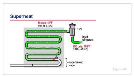
The TXV meters refrigerant by measuring the condition of the refrigerant vapor leaving the evaporator. **Superheat** is the additional heat absorbed by the refrigerant in the evaporator after it has completely vaporized. It provides a safety factor by preventing liquid refrigerant from entering the compressor.
