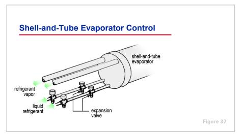
The capacity of a shell-and-tube evaporator is primarily controlled by the unloading or cycling of compressors. However, as with a finned-tube evaporator, it also uses an expansion valve to control the flow rate of refrigerant through the evaporator and ensure the proper amount of superheat in the system.
