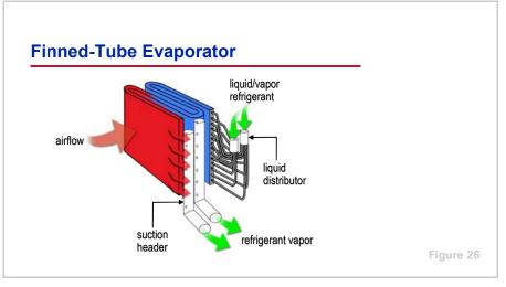
To provide uniform heat transfer throughout the coil, the liquid refrigerant is distributed to the coil tubes in several parallel circuits. A **distributor** is used to ensure uniform refrigerant distribution through these multiple coil circuits. It distributes the liquid/vapor refrigerant mixture to the coil through several tubes of equal length and diameter.
