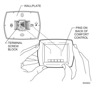
**5.** Push the comfort control straight onto the wallplate until it snaps into place.
