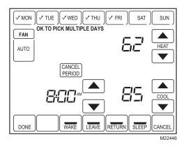
NOTE: Note that the time, temperature(s) and fan setting disappear. The bar above the selected period is removed, indicating the scheduled period was cancelled. To reinstate a schedule period, press arrow keys to set desired time and temperatures.
