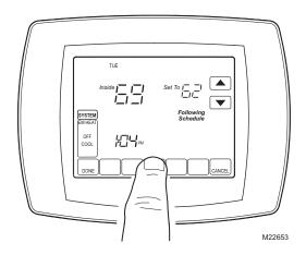
3. Release the center key when the display on your comfort control matches the display below.
