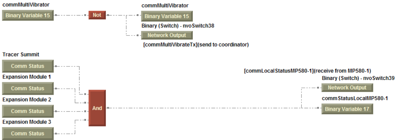
Figure 65. Collection of Tracer and EX2 communication status at an individual MP581
