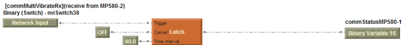
Figure 64. Sample TGP showing watchdog signal receive process
