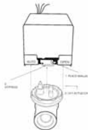
Figure 12: Removing valve actuator
