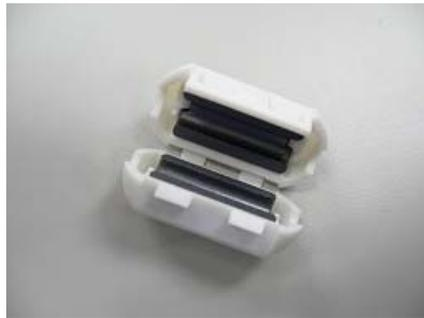
2. Place the EMI core as close as possible to the earphone jack. Loop the earphone cable around the core to ensure a snug fit. Close the core and press tightly on the core's fasteners.
