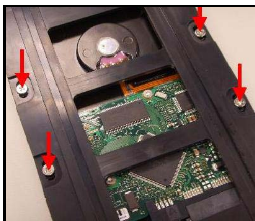
Figure 6. Secure the hard drive to the panel using the provided screws
