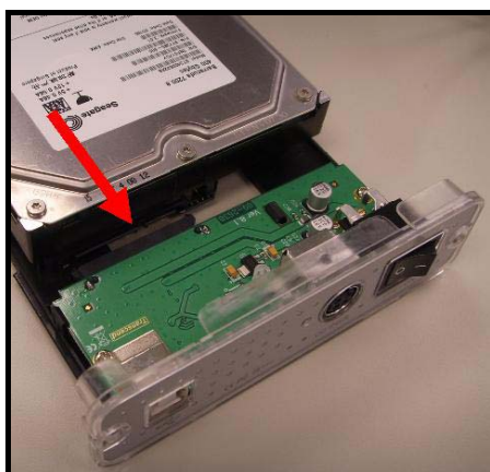
Figure 5. Connect the SATA hard drive to the SATA adapter
