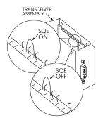
If connecting the Coaxial Transceiver to a terminal device, set the SQE jumper to ON by
