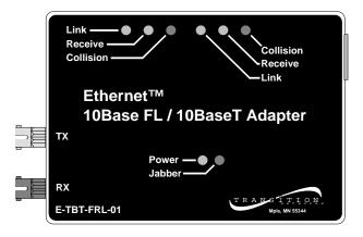
The 10BaseFL/10BaseT Adapter provides an RJ-45 twisted pair connector and a set of Receive and Transmit ST fiber optic connectors. The twisted pair connection allows a 10BaseT device to be located at a distance of up to 100 meters (185 feet). The fiber optic ST connections allows a device to be located at a distance of up to 2000 meters (6,600 feet). NOTE: A media converter with an SMA type fiber connection, E-TBT-FRL-01(SMA), also is available.
