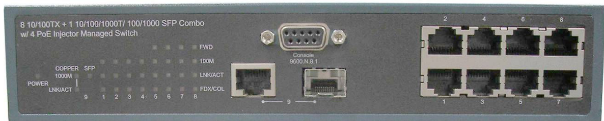
The Front panel of the 8 10/100TX + 1 10/100/1000T/100/1000 SFP Combo with 4 PoE Injectors Managed Switch
